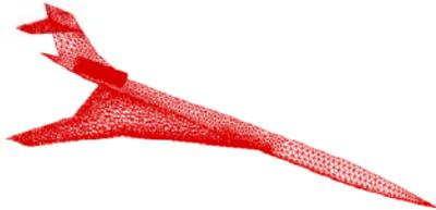
Fig.1 Surface triangulation of baseline configuration
