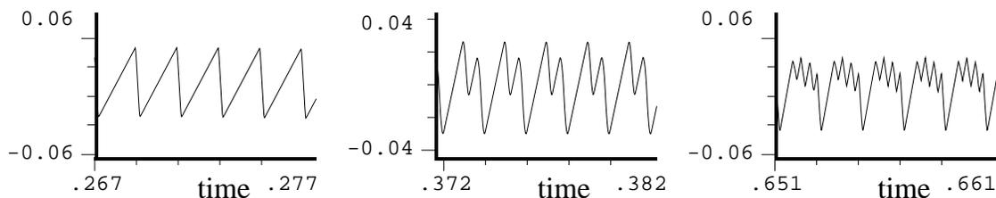
Figure 1: Helmholtz String Displacement. a) Ideal motion. b) multiple slips. c) chaotic motion
